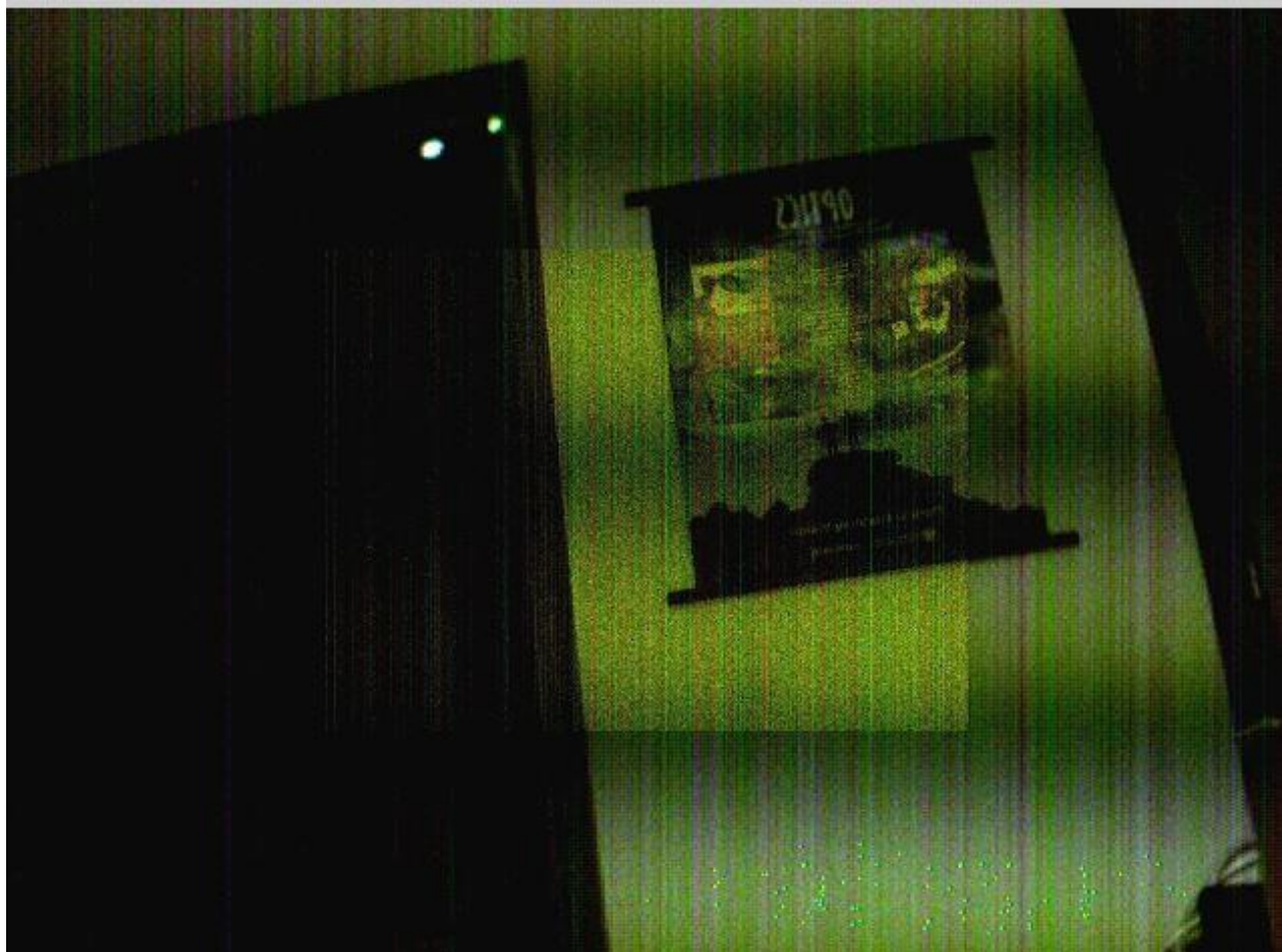
Figure 6.2.1-4 FPN presented when the imager operates at high frame rates.
