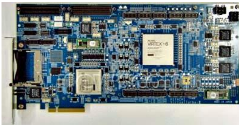
Figure 2.7.2-1 Xilinx Vertex 6 FPGA with a PCI-X communication for fast image data transmission.
